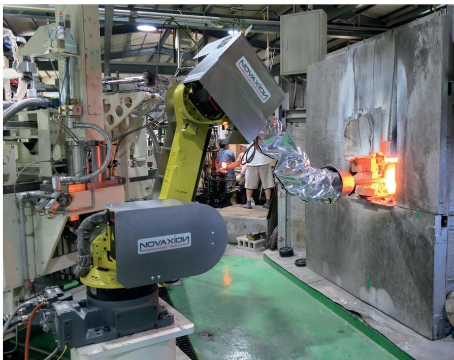
breakdown or production change causes important glass losses. With a slow speed there is a necessity to flow down a glass trickle and to make a pre-gob before being able to get the right gob. So there is less flexibility with a gob feeder.
