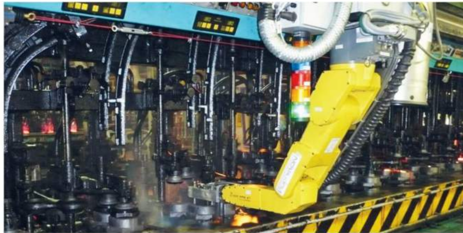
▲ Picture 1. First hanged-up Swabbing Robot in 2011 in Saint-Gobain Oberland, Germany.
